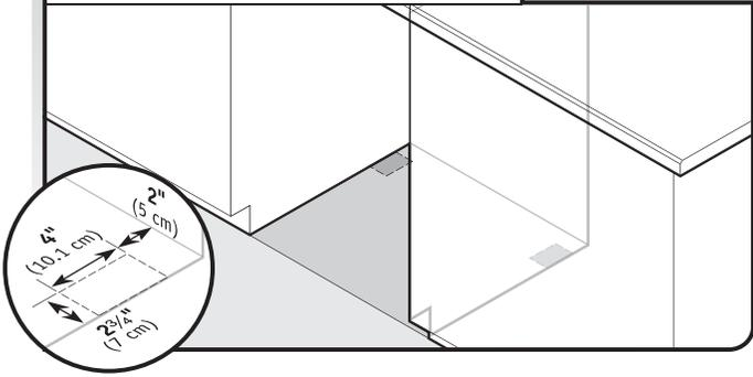
**Built-up floors:** If the kitchen floor is higher than the cabinet opening's floor - for example, the kitchen floor tile does not extend into the cabinet opening - add shims as needed in the area shown to bring the dishwasher up to 33½" (85.1 cm) below the countertop.
