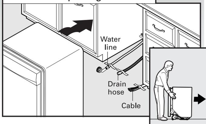
**IMPORTANT:** Double-check correct placement of utilities. Grasp the sides of the dishwasher at the edges of the door panel. Move dishwasher close to cabinet opening.
