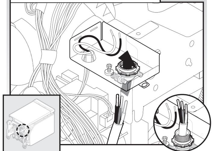
Route cord so that it does not touch dishwasher motor to lower part of dishwasher tub. Pull cord through strain relief in terminal box.
