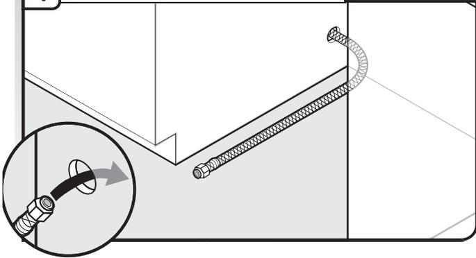
Slowly route water supply line through hole in cabinet. (If you are using copper tubing, it will bend and kink easily, so be gentle.) It should be far enough into the cabinet opening to connect it to the dishwasher inlet on the front left side of the dishwasher.
