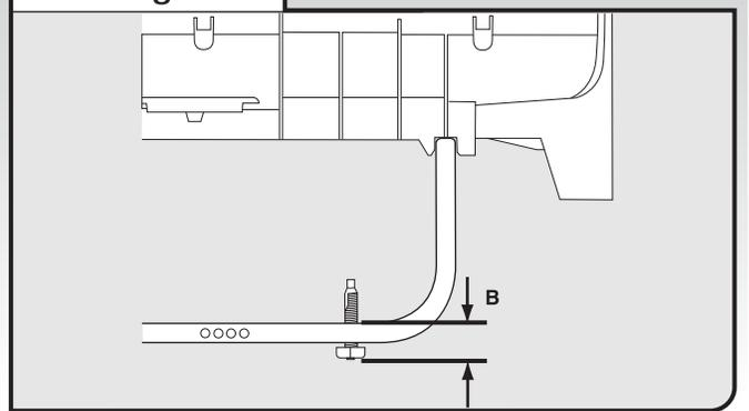
**NOTE:** If the minimum cabinet opening height is less than 33 7⁄8" (86 cm), the rear leveling legs and spacers can be removed for additional clearance. This will allow the dishwasher to fit into a 33 1⁄2" (85.1 cm) high cabinet opening, but the dishwasher will be more difficult to move. (Measurements are approximate. Rear and front leveling legs are preset at the factory for 34 1⁄2" [87.6 cm].)
