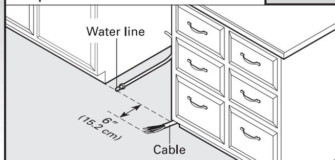
If the water line and the cable extend to the locations shown, proceed to the “Install Drain Hose” section. If they do not reach far enough, follow the instructions in the “Prepare Cabinet Opening—New Utilities” section.
