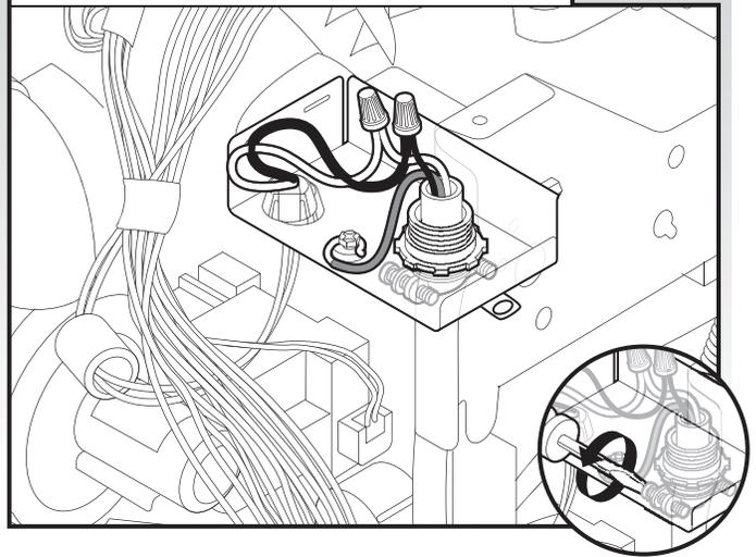
Tighten strain relief screws to secure cord.
