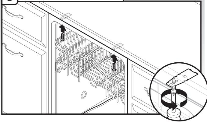
**NOTE:** Do not drop screws into bottom of dishwasher. Locate brackets on top of dishwasher and secure dishwasher to countertop with two, #10 x 1/2" Phillips-head screws (included). The dishwasher must be secured to keep it from shifting when door is opened.
