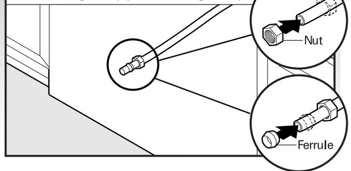
Copper tubing only: Slide nut, then ferrule, about 1" (2.5 cm) onto copper tubing.
