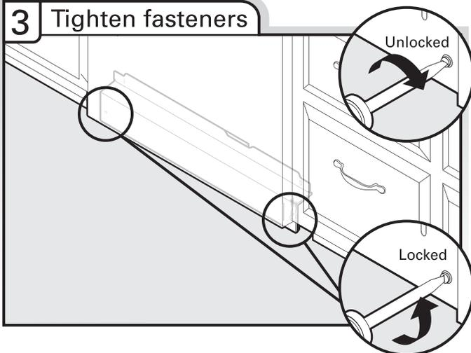
Using a flat-blade screwdriver, turn the fasteners  $\frac{1}{4}$  turn to lock into place. The fasteners slot will be straight up and down when properly locked.
