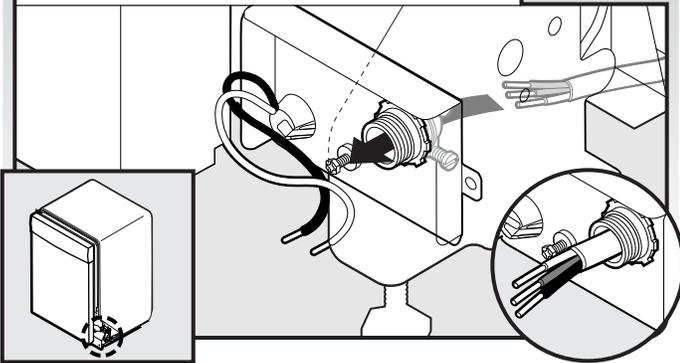
Route cable so that it does not touch dishwasher motor or lower part of dishwasher tub. Pull cable through UL Listed/CSA Approved strain relief in terminal box. Strain relief is not supplied with the dishwasher. Owner must purchase a  $\frac{3}{8}$ " screw-in type strain relief.
