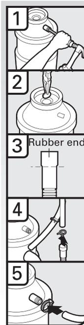
1. Using a hammer and screwdriver, knock plug into disposer.
