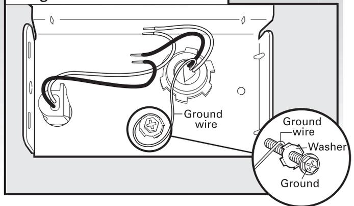
Form bare ground wire into a U-shaped hook. Wrap ground wire hook clockwise around ground connector screw and under the washer. Securely tighten ground connector screw.
