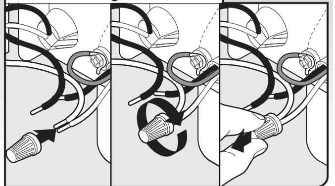
**NOTE:** Do not pre-twist stranded wire. Twist on UL listed/CSA approved wire connector. Gently tug on wires to be sure both are secured.
