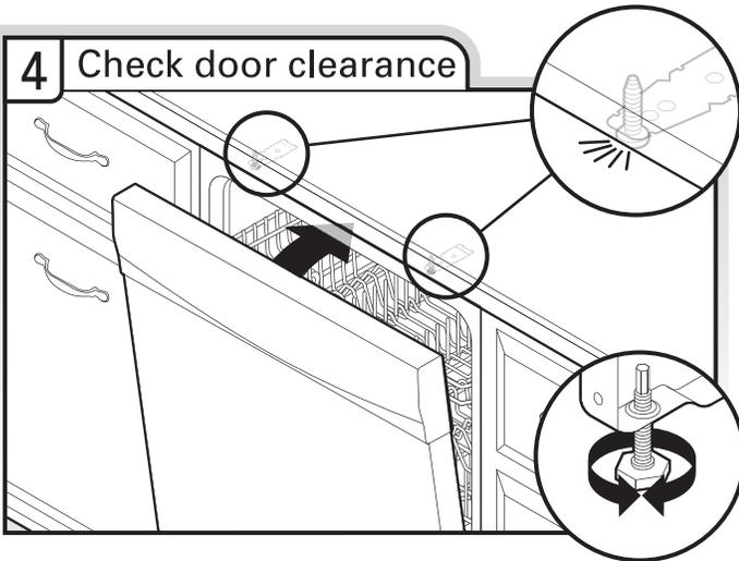
Check that top of door does not contact screws, brackets or countertop. If it does, adjust leveling legs.
