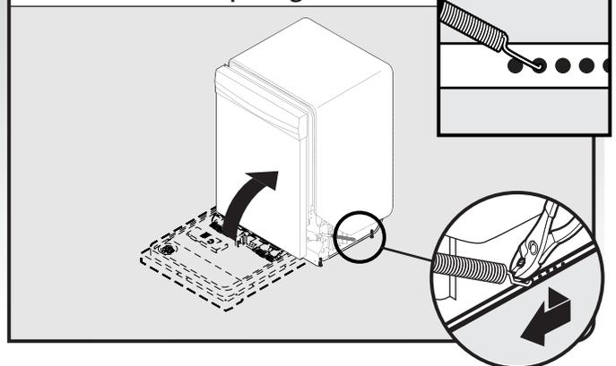
If the door closes too quickly, decrease the spring tension by moving the spring end toward the front of the dishwasher.
