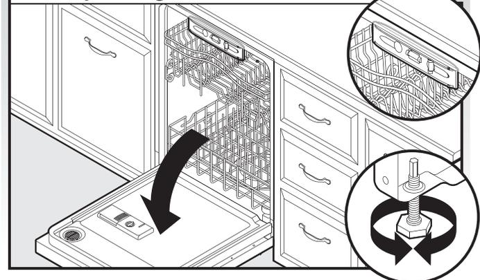
Place level against top front opening of tub. Check that dishwasher is level from side-to-side. If dishwasher is not level, adjust front legs up or down until dishwasher is level. Close the dishwasher door.
