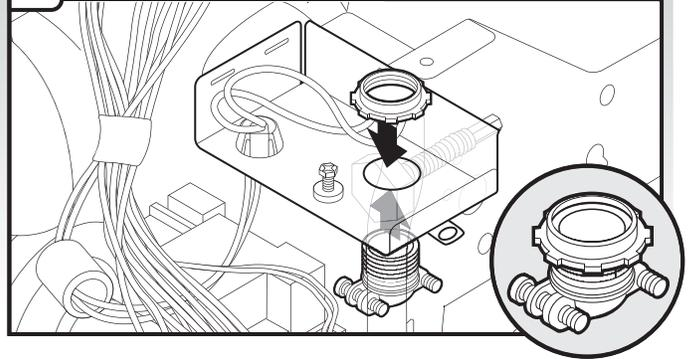
Install a UL Listed/CSA Approved strain relief. Make sure screw heads are facing to the left when tightening conduit nut. Strain relief is provided with the power supply cord kit.
