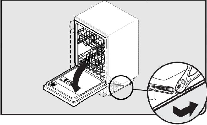
If the door falls open, increase the spring tension by moving the spring end toward the back of the dishwasher.
