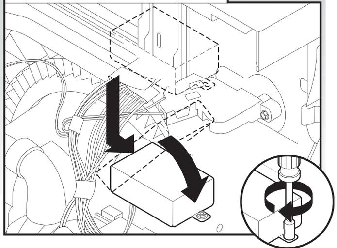
Place wires inside terminal box. Insert tabs on left side of cover. Make sure wires are tucked inside box. Close cover ensuring wires are not pinched. Use 1/4" nut driver or Torx® T20® screwdriver and previously removed screw to secure cover.
