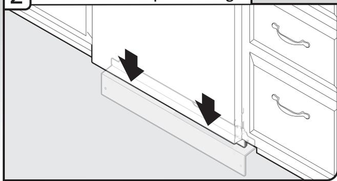
Check that the lower edge of the access panel touches the floor. Adjust if necessary.
