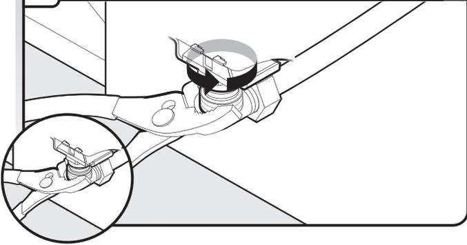
Be sure rubber washer is properly seated in fitting. Slide the  $\frac{3}{4}$ " fitting up to the valve and hand tighten to avoid cross-threading. Hand tighten until the coupling is tight.
