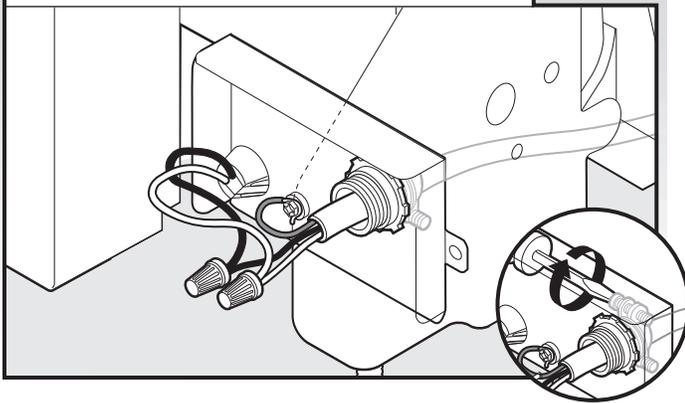
Tighten strain relief screws to secure cable.
