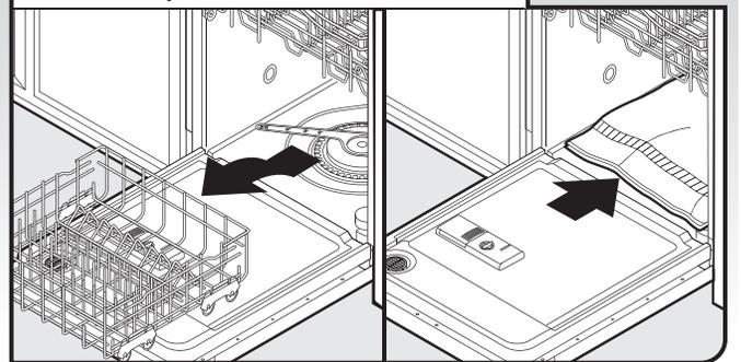
Open dishwasher door, remove lower dish rack, and place towel over pump assembly and lower spray arm of dishwasher. This will keep screws from falling into pump area when you are securing the dishwasher.
