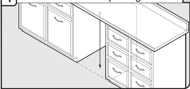
Measure height of cabinet opening from underside of countertop to floor where dishwasher will be installed (you will need to measure the lowest point on the underside of the countertop and the highest point on the floor). Refer to "Dishwasher Height Adjustment Chart" to adjust the leveling legs.
