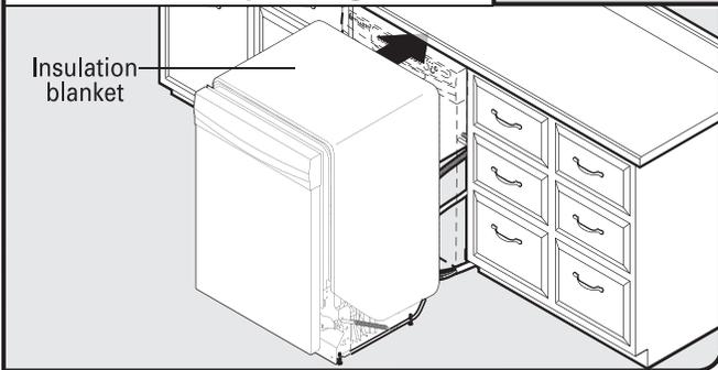
**IMPORTANT:** If rear leveling legs and spacers were removed, cover the floor when moving the dishwasher to avoid damage to the floor. Slowly move dishwasher completely into cabinet opening. Do not kink or pinch water line, drain hose, power supply cord or direct wire between dishwasher and cabinet. Remove cardboard from under dishwasher.
