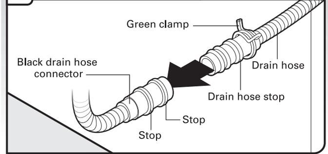
Place towel under drain hose to catch any water in drain hose. Place the small drain hose clamp onto the small end of the drain hose. Push the new drain hose into the black drain hose connector up to the drain hose stop.
