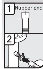
1. Fit rubber end of drain hose to waste tee and cut if needed.
