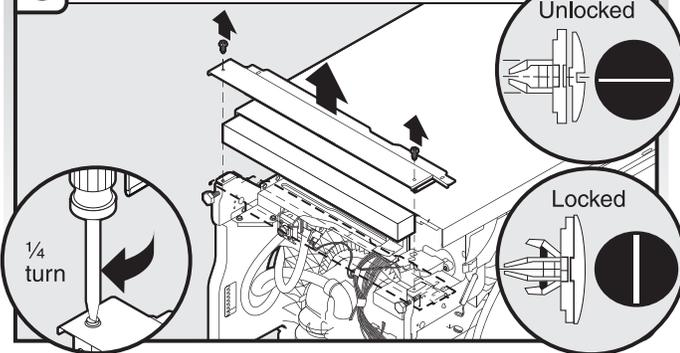
Using a flat-blade screwdriver, turn the plastic fasteners  $\frac{1}{4}$  turn to unlock them. Remove panel. Do not remove tech sheet from access panel.
