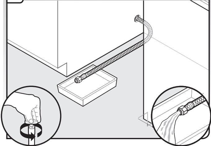
Slowly turn water shutoff valve to "ON" position. Flush water into a shallow pan until clear to get rid of particles that could clog the inlet valve. Turn shutoff valve to "OFF" position.
